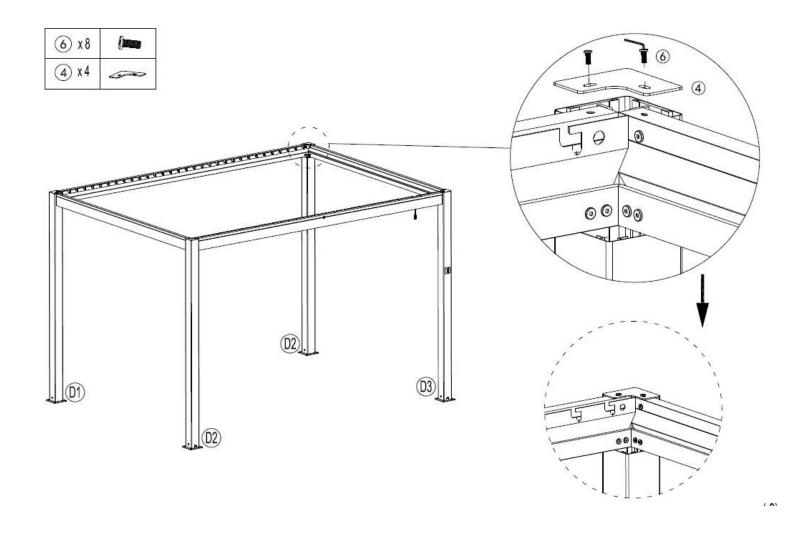
Step 5 Attach all four gutters ( x2 and x2 )by hooking inside the , , beams
